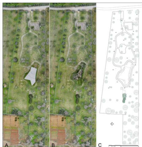
The 3D survey: (A), the digital aerial photogrammetry of the archaeological site; (B), the aerial survey merged with the digital close range photogrammetry; (C), CAD plan.
